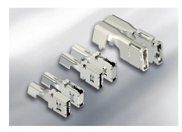
The new line of terminals, PCON 12, PCON 18 and PCON 21, have a common body design optimized for maximum vibration resistance while minimizing mating forces. Each is available with 90° and 180° mating directions and accommodates wire sizes ranging from 5 mm² to 95 mm² supporting continuous currents up to 400 Amps.
