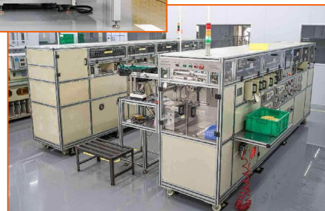
Automatic electrical performance testing line
