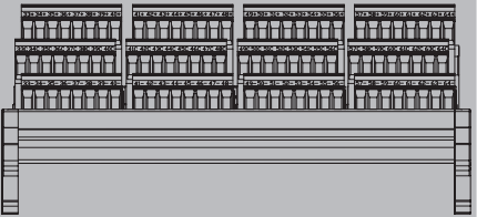
Field terminals view for ADV161 (Channels 33 to 64)
