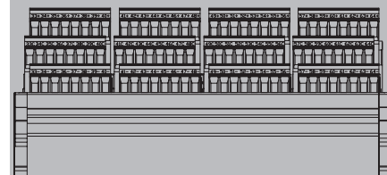
Field terminals view for ADV161 (Channels 33 to 64)
