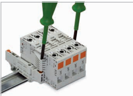
Removing the assembly: Insert two operating tools into the separator slots between male and female connectors and unlatch the assembly.
