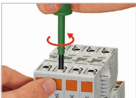
Insert operating tool and turn counterclockwise. Then push in orange locking tab for handsfree wiring.
