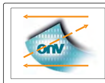
Fig. 2 Reverse scan (Pin24, Reverse = High)
